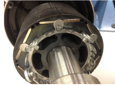
Figure 2. Rotor of the IPMSM motor with shifted stacks.
