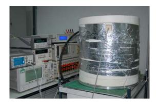
Figure 11. Measurement system of the calorimeter.
