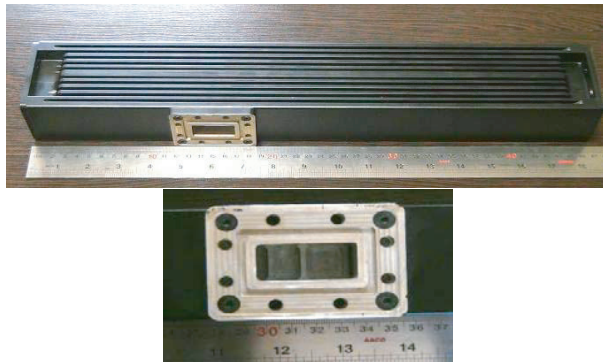
Figure 6. Fabricated E -plane waveguide diplexer.
