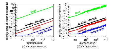
**Figure 3.** Averaged relative error of the analytically computed rectangle potential (Refs. [26, 27], (a) and rectangle field (Ref. [19], (b) as a function of the distance ratio, for float (green), double (red) and long double (blue) C++ arithmetic types (with low aspect ratio rectangles), and with double precision and high aspect ratio (AR = 200) rectangles (black).
