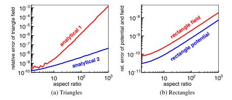
**Figure 4.** Averaged relative error of the analytically computed triangle field (a), 1 (red): Ref. [19], 2 (blue): Ref. [26]), and rectangle potential and field (b), Ref. [26]; Ref. [19] is similar), as a function of the aspect ratio, with fixed distance ratio DR = 300.
