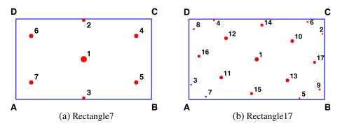
**Figure 7.** Gaussian points of the 7-point (a) and the 17-point (b) cubature formula for rectangle. The numbers are the indices of the Gaussian points. The surfaces of the red circles are proportional to the corresponding weights.
