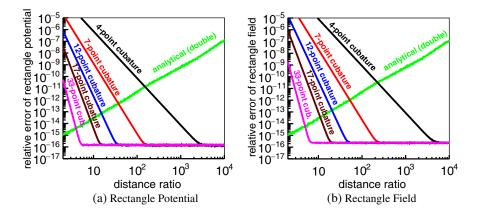
**Figure 9.** Averaged relative error of the rectangle potential (a) and field (b) for the 5 Gaussian cubature approximations of App. B, as a function of the distance ratio. For comparison, the averaged relative error of the rectangle potential and field computed by analytical integration (Refs. [26, 27]) is also shown.
