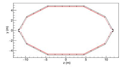
Figure 11. Schematic cross-sectional view of the KATRIN main spectrometer vessel (black, outside) and inner electrode system (red, inside).
