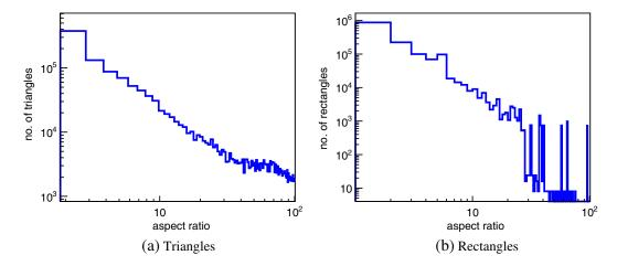
**Figure 12.** Aspect ratio distribution of triangles (a) and rectangles (b) of our two discretization models of the KATRIN main spectrometer electrode system with electric dipole field. Vertical axis: number of elements per bin, with constant bin size 1.
