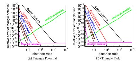
**Figure 8.** Averaged relative error of the triangle potential (a) and field (b) for the 5 Gaussian cubature approximations of App. A, as a function of the distance ratio. For comparison, the averaged relative error of the triangle potential and field computed by analytical integration (Refs. [26, 27]) is also shown.
