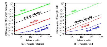
**Figure 2.** Averaged relative error of the analytically computed triangle potential (Refs. [19, 25], (a) and triangle field (Refs. [26, 27], (b) as a function of the distance ratio, for float (green), double (red) and long double (blue) C++ arithmetic types (with low aspect ratio triangles), and with double precision and high aspect ratio (AR = 200) triangles (black).
