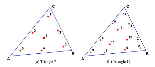
**Figure 6.** Gaussian points of the 7-point (a) and the 12-point (b) cubature formula for triangle. The numbers are the indices of the Gaussian points. The surfaces of the red circles are proportional to the corresponding weights.
