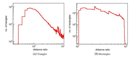
**Figure 13.** Distance ratio distribution of triangles (a) and rectangles (b) of our two discretization models of the KATRIN main spectrometer electrode system with electric dipole field, at field point  $\mathbf{P} = (0,0,0)$  (center of spectrometer). Vertical axis: number of elements per bin, with constant bin size 10.
