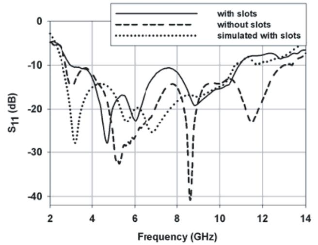
Figure 11. Return loss of fabricated antenna.
