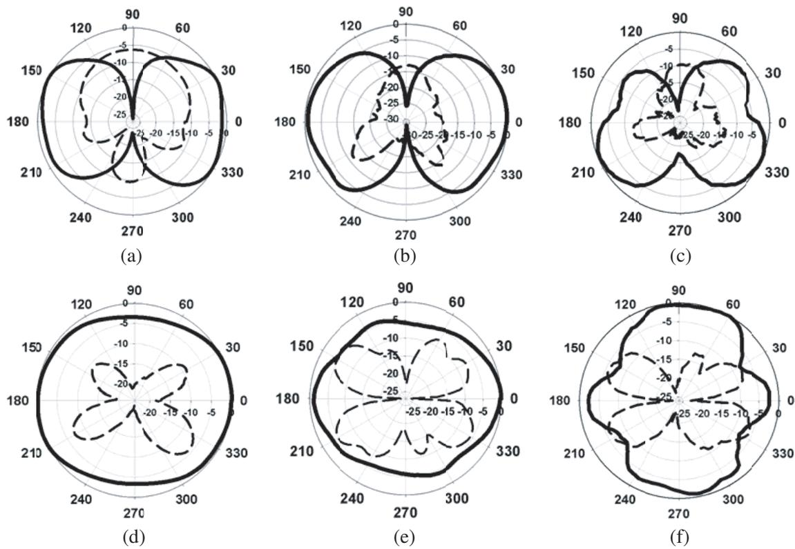
Figure 9. Radiation pattern of unique antenna [3], co-polarised (solid line), cross polarised (dashed line). (a) *E*-plane (4 GHz). (b) *E*-plane (7 GHz). (c) *E*-plane (10 GHz). (d) *H*-plane (4 GHz). (e) *H*-plane (7 GHz). (f) *H*-plane (10 GHz).
