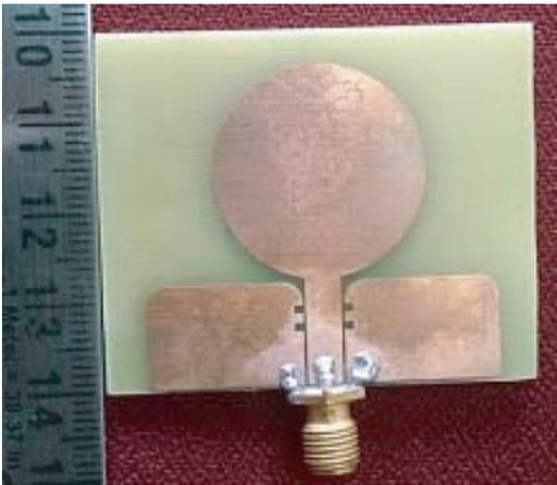
Figure 10. Circular monopole antenna.
