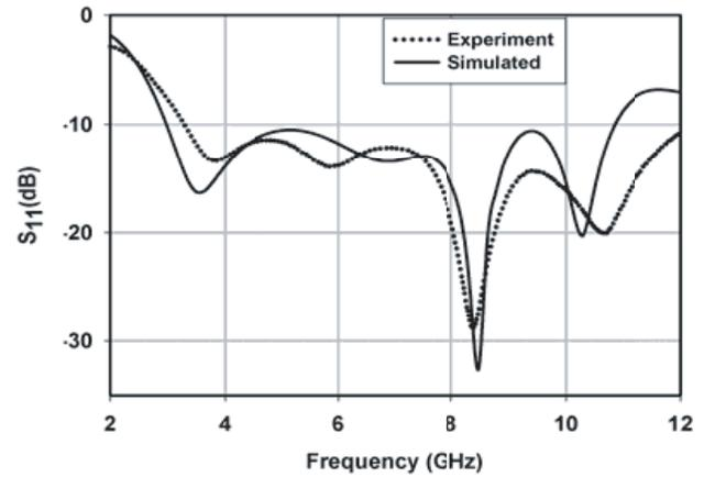
Figure 8. Return loss of fabricated antenna.
