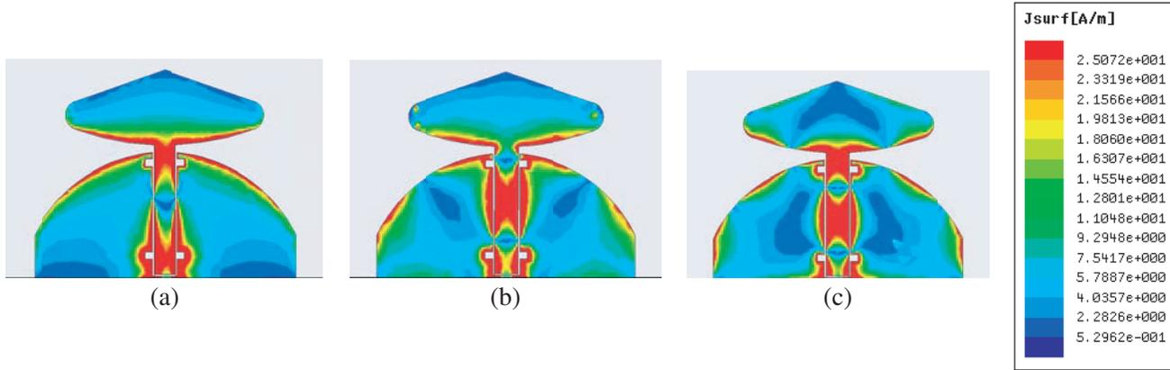
**Figure 5.** Simulated current density of the unique antenna. (a) 3.6 GHz. (b) 8.5 GHz. (c) 10.3 GHz.
