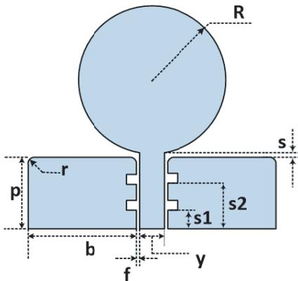
**Figure 3.** Circular monopole with slots.
