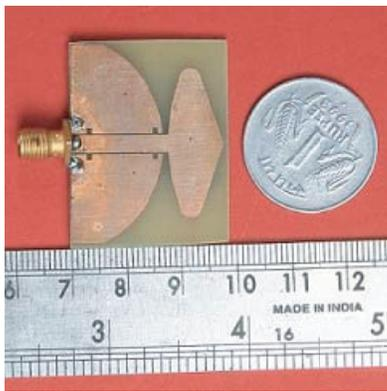
Figure 7. Fabricated antenna.
