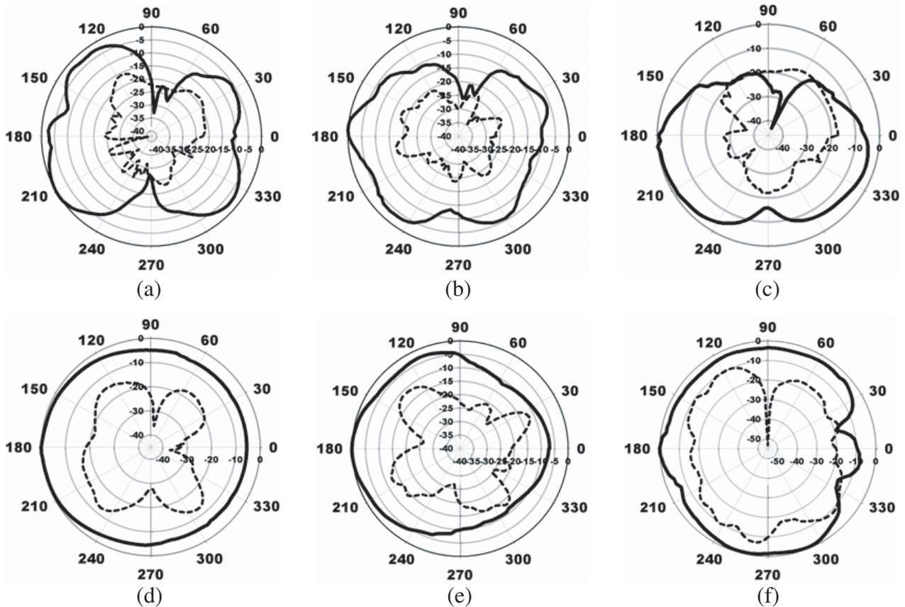
Figure 12. Radiation pattern of the circular monopole with slots in MGP, co-polarisation (solid line), cross-polarisation (dashed line). (a) *E*-plane (4 GHz). (b) *E*-plane (7 GHz). (c) *E*-plane (10 GHz). (d) *H*-plane (4 GHz). (e) *H*-plane (7 GHz). (f) *H*-plane (10 GHz).
