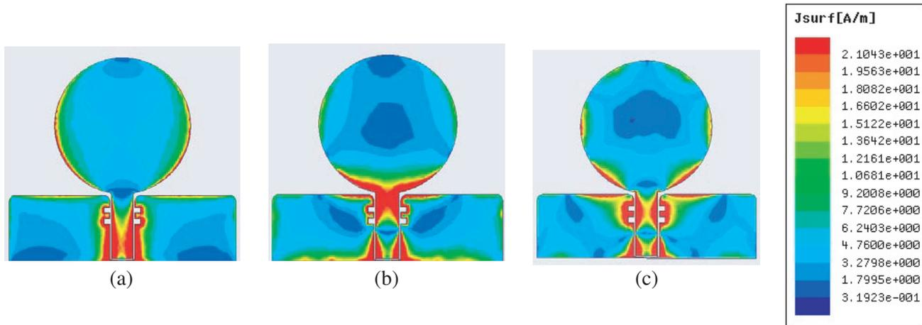
**Figure 6.** Simulated current density of circular monopole. (a) 3.4 GHz. (b) 6.8 GHz. (c) 10.2 GHz.
