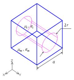
Figure 1. Unit cell of the metamaterial.
