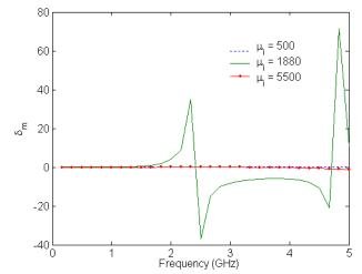
Figure 4. Real part of  $\mu_{eff}$  of metamaterial versus frequency  $\omega$  of LHCP wave propagated in direction of bias.
