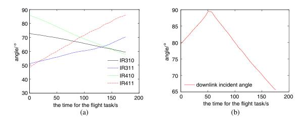
**Figure 7.** Incident angle of the EM wave: (a) between the vehicle and the potential satellites (uplink); (b) between the vehicle and the ground station (downlink).
