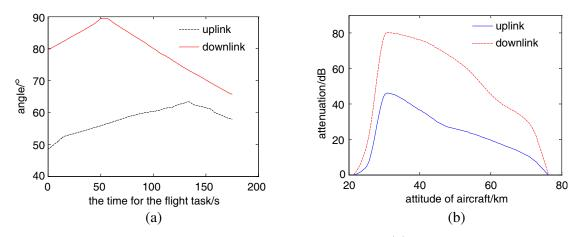
Figure 10. Comparison between the uplink and the downlink: (a) incident angle of EM wave; (b) attenuation.
