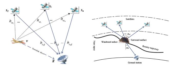
Figure 1. Schematic diagram of a LEO relay communication for hypersonic vehicles versus downlink direct communication.
