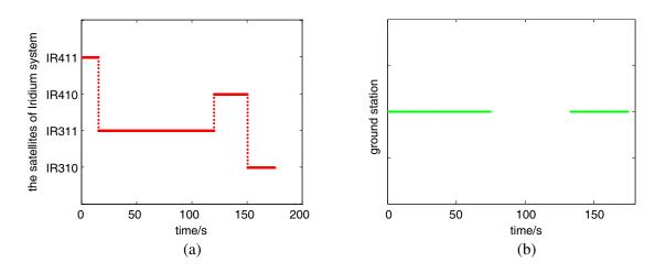
Figure 9. Coverage performance comparison: (a) proposed relay strategy with LEO; (b) direct communication with the ground station.
