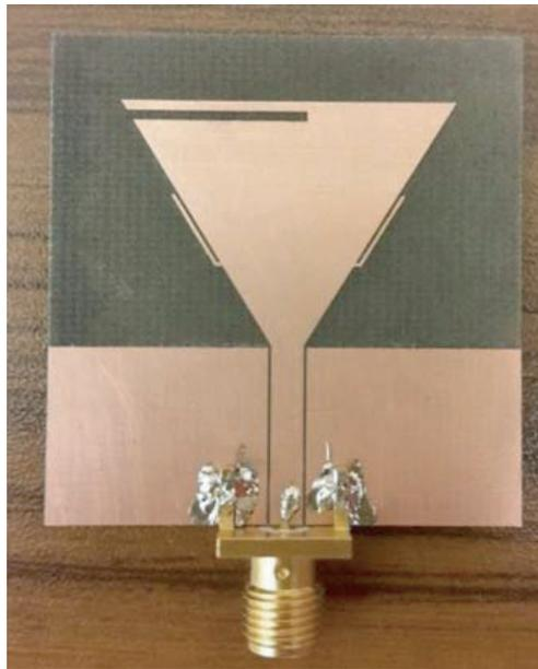
**Figure 5.** Fabricated prototype of the proposed antenna.
