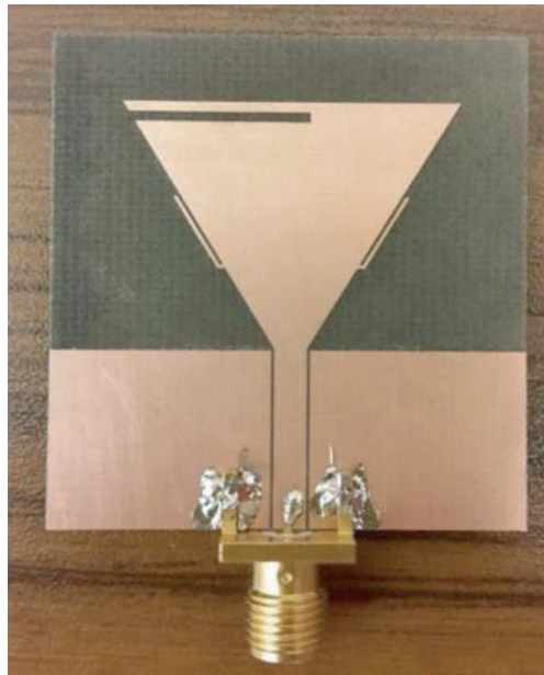
Figure 5. Fabricated prototype of the proposed antenna.
