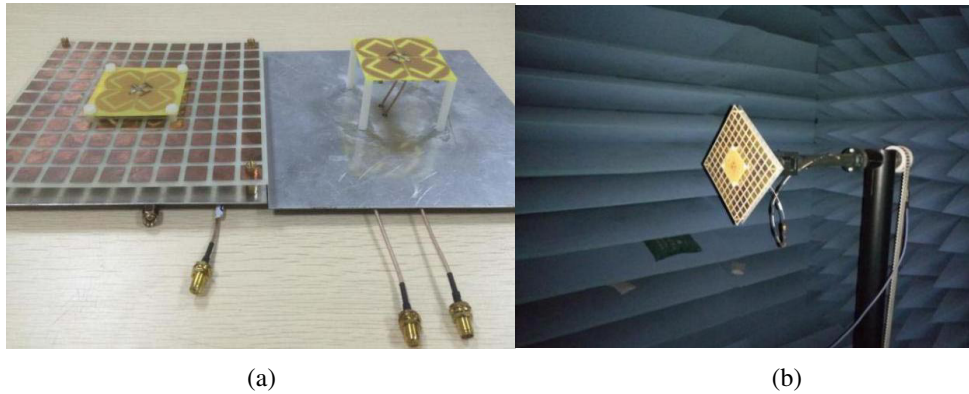
Figure 7. The fabricated antenna and testing environment. (a) Comparison of the antenna with an AMC reflector and the same antenna with a PEC reflector. (b) The testing environment.
