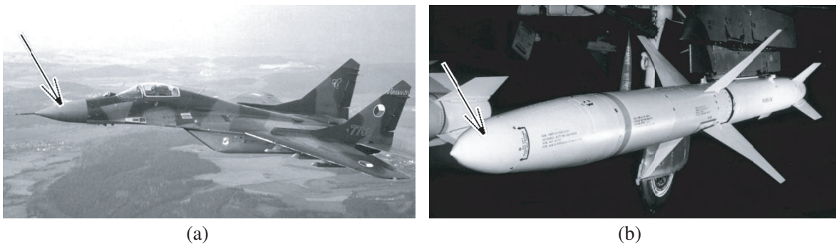
Figure 1. Use of antenna systems under dielectric radomes by (a) aircrafts and (b) missiles.
