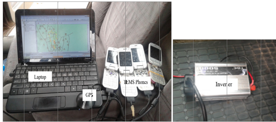
Figure 1. Drive test tools housed in a vehicle.
