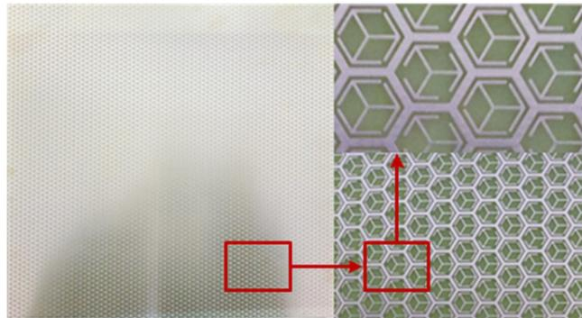
**Figure 5.** Photograph of the fabricated miniaturized FSS.
