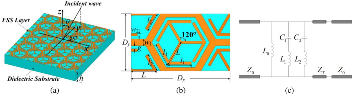
**Figure 1.** Structure of the proposed FSS structure and its equivalent circuit model. (a) Three dimensional view. (b) The unit cell. (c) Its transmission line model.
