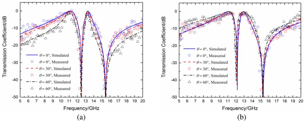
**Figure 6.** Comparisons between simulated and measured results. (a) TE polarization. (b) TM polarization.
