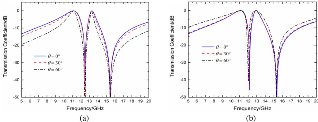
**Figure 4.** Transmission coefficients of the proposed FSS structure under oblique incidence. (a) TE polarization. (b) TM polarization.
