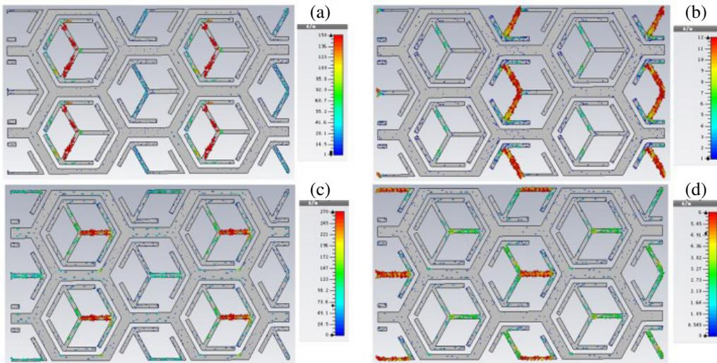
**Figure 3.** Surface current distribution of the proposed FSS for TE ((a) and (b)) and TM ((c) and (d)) polarization: (a) (c) At  $f_{z1}$ , (b) (d) At  $f_{z2}$ .
