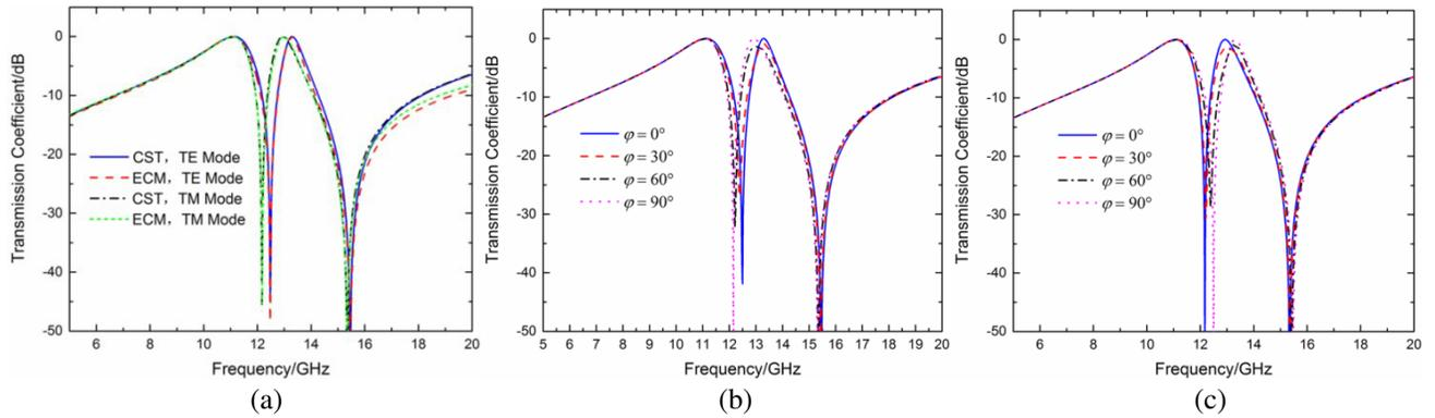
**Figure 2.** Transmission coefficient of the proposed FSS at normal incidence (a) With polarization angle  $\varphi = 0^\circ$ . (b) With different polarization angles for TE polarization. (c) With different polarization angle for TM polarization.
