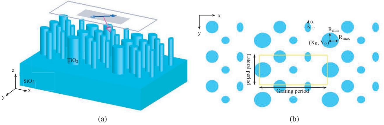
**Figure 1.** (a) Three dimensional schematic of a beam deflector made of extended unit-cells containing TiO<sub>2</sub> nano elliptical antennae on fused silica substrate. (b) Design parameters of the extended unit-cell. The yellow line shows the boundaries of the extended unit-cell.
