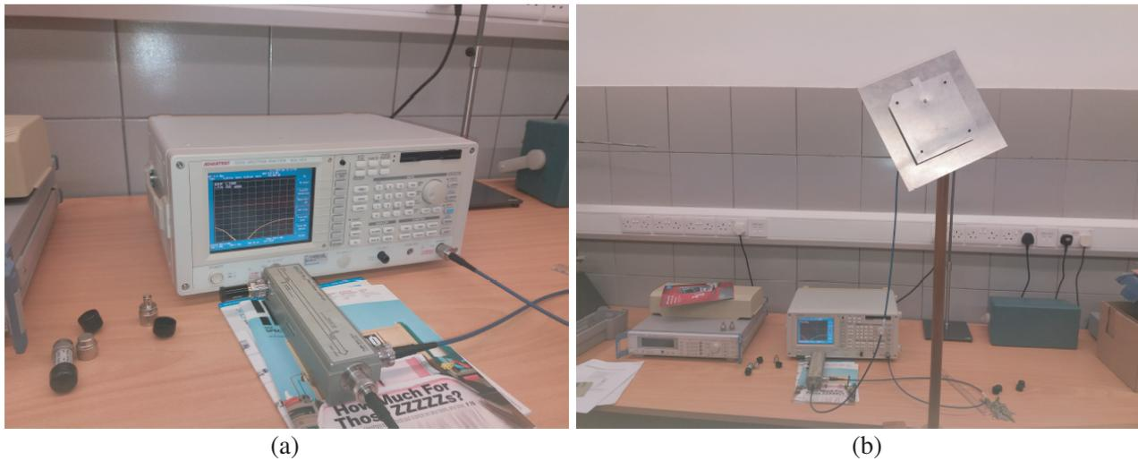
**Figure 7.** Measurement setup for the single-patch antenna. (a) Spectrum analyzer and directional coupler; (b) Spectrum analyzer, directional coupler and antenna.
