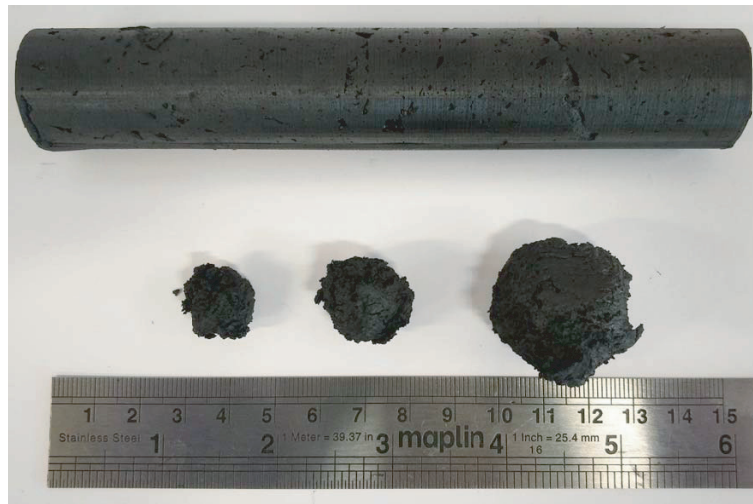
Figure 6. Haemorrhagic phantom lesions (bottom) are shown alongside an example of a completed cylindrical phantom tissue plug (top). These plugs are either made wholly of the brain mimicking TMM or have a haemorrhagic phantom lesion embedded in them at a known location. Haemorrhagic phantom lesions can be of any size or shape as long as they fit within the dimensions of the cylindrical plug. These plugs are fitted into the cavities in the brain part of the head phantom to complete it.
