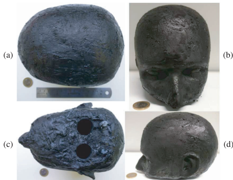
Figure 7. Photograph of the fabricated dielectrically and anatomically realistic head phantom. The phantom contains two 25 mm diameter cylindrical hollows bilaterally located across the sagittal plane along with a symmetrically placed circulatory loop across the midline. The head phantom is shown upright ((a), (b) and (d)) and inverted ((c)). The inverted view shows the two cylindrical cavities, which can be filled with phantom plugs, as well as the entry and exit points of the rubber tubing used to create the circulatory loop. The loop forms an arc with the apex reaching approximately half way into the brain cavity.
