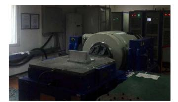
Figure 7. Electrical shaking table.
