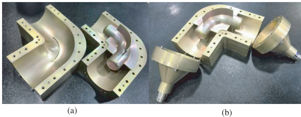
Figure 11. Photograph of (a) bent CWG and (b) cascade of bent CWG and two impedance and mode converters.
