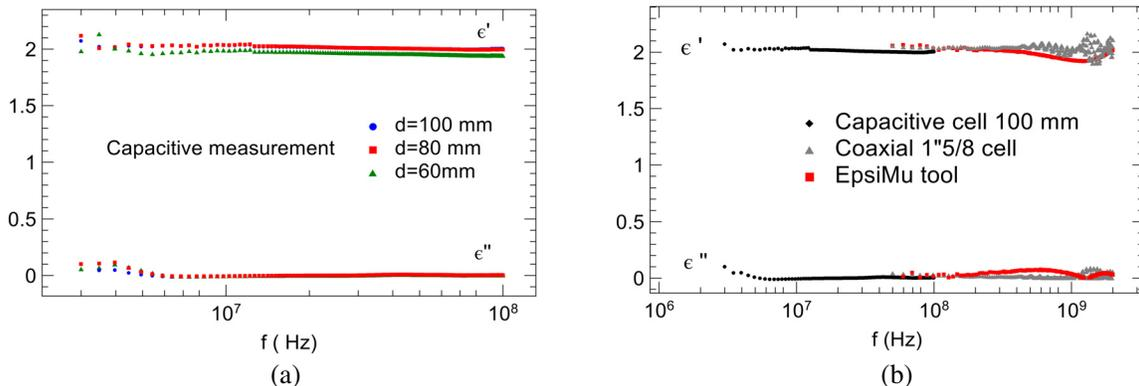
**Figure 3.** PTFE: (a) Sample diameter effect, (b) permittivity result with different instruments.
