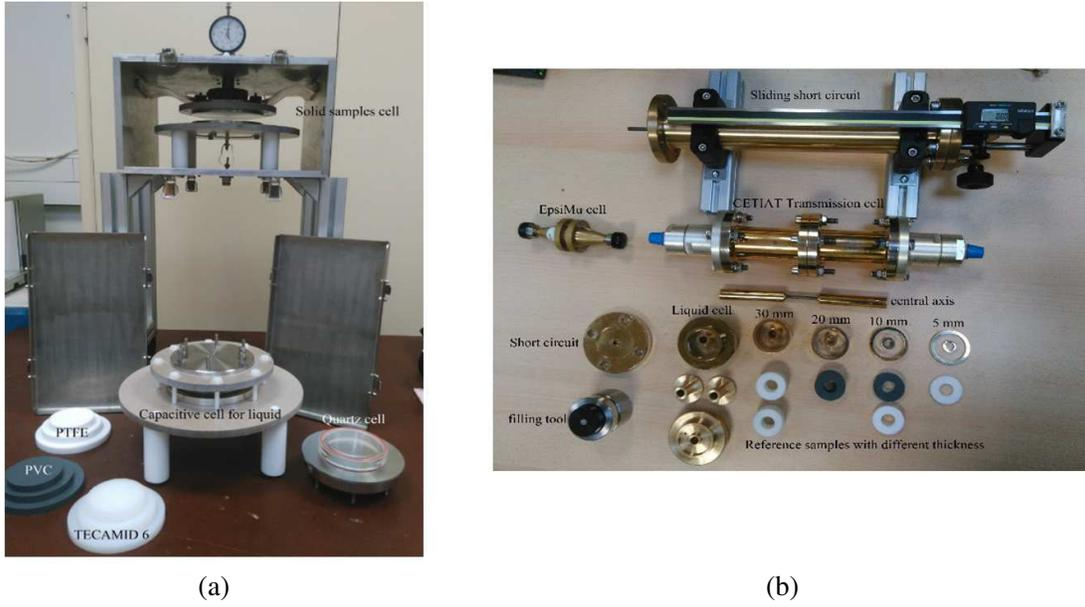
**Figure 1.** (a) Capacitive cell, (b) coaxial cells with sample holders for solids and liquids.
