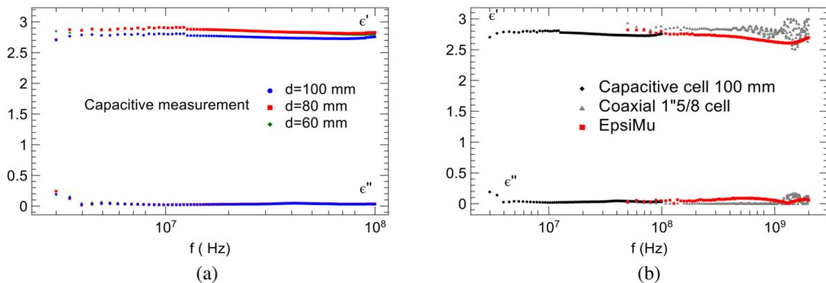
Figure 4. PVC: (a) Sample diameter effect, (b) permittivity result with different instruments.
