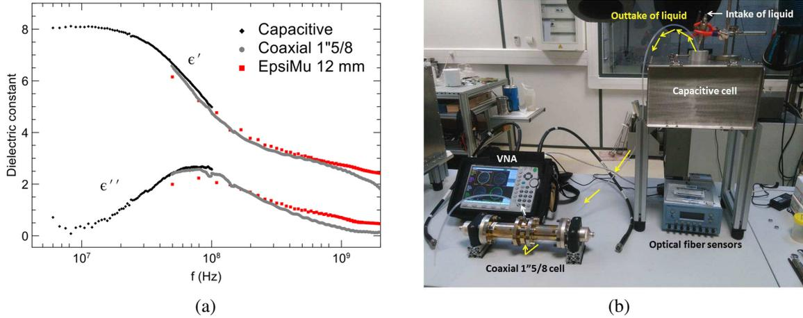
**Figure 2.** Decanol at 25°C: (a) Measurement results, (b) experimental liquid manipulation.
