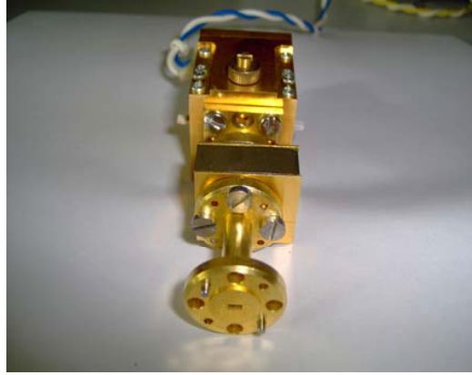
Figure 5. A photograph of avalanche diode high order frequency multiplier.
