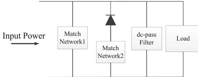
**Figure 1.** Topological structure of the proposed rectifier.
