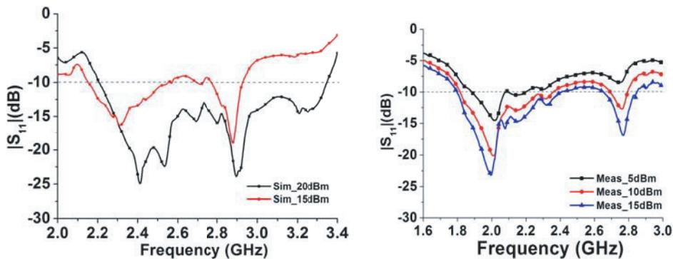
**Figure 7.** Simulated and measurement  $|S_{11}|$  of the rectifier.
