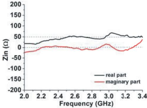
**Figure 3.** Simulated input impedance  $Z_{in}$  vs. frequency.
