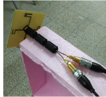
Figure 7. Environment set-up for the impedance measurement of the cross-dipole tag antenna.
