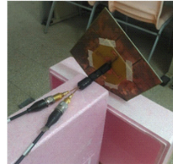
Figure 13. Impedance measurement of the cross-dipole tag together with the 3 \times 3 AMC substrate.
