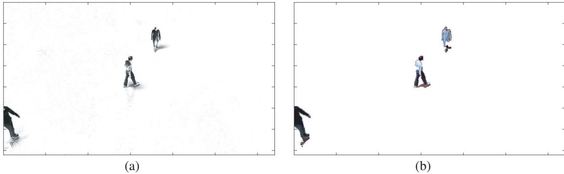
**Figure 4.** Grayscale image motion detection results. (a) Motion detection result  $C_I$ . (b) Moving objects extracted from the scene.
