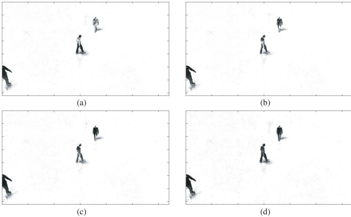
**Figure 5.** Motion detection results of RGB color image via HQ minimization. (a) Motion detection result of  $R$  channel. (b) Motion detection result of  $G$  channel. (c) Motion detection result of  $B$  channel. (d) Motion detection fusion result.
