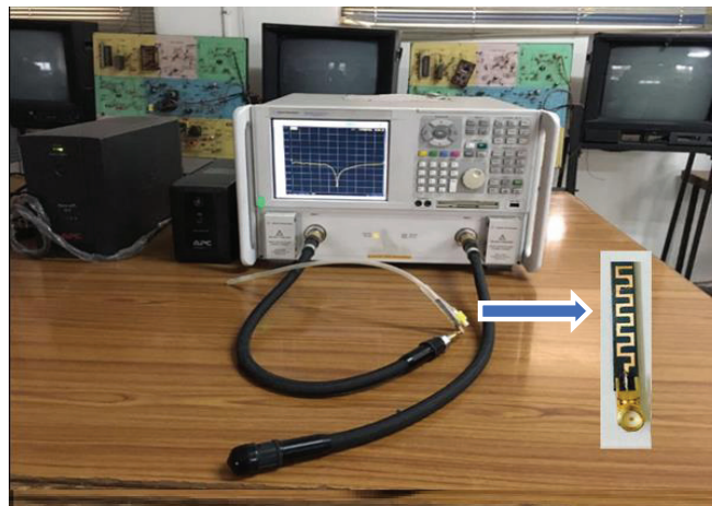
Figure 11. Measurement in silicone feeding tube using VNA.
