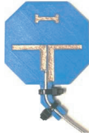
Figure 15. Yagi-Uda antenna with copper radiators.
