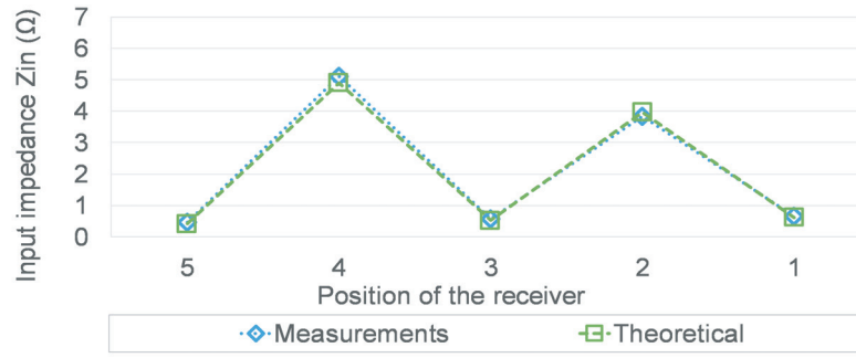
Figure 7. \hat{Z}_{in}(\Omega) at the resonant frequency f_0 = 147 kHz obtained with measurement using the VNA and with Eq. (6) using Eq. (3) versus different positions of the receiver.
