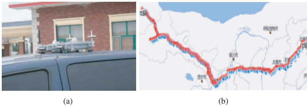
Figure 9. (a) Photo of the vehicle antenna prototype; (b) measured trajectory and map route of the test travel.
