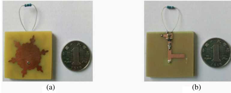
Figure 16. The photograph of rectenna: (a) top view, (b) bottom view.
