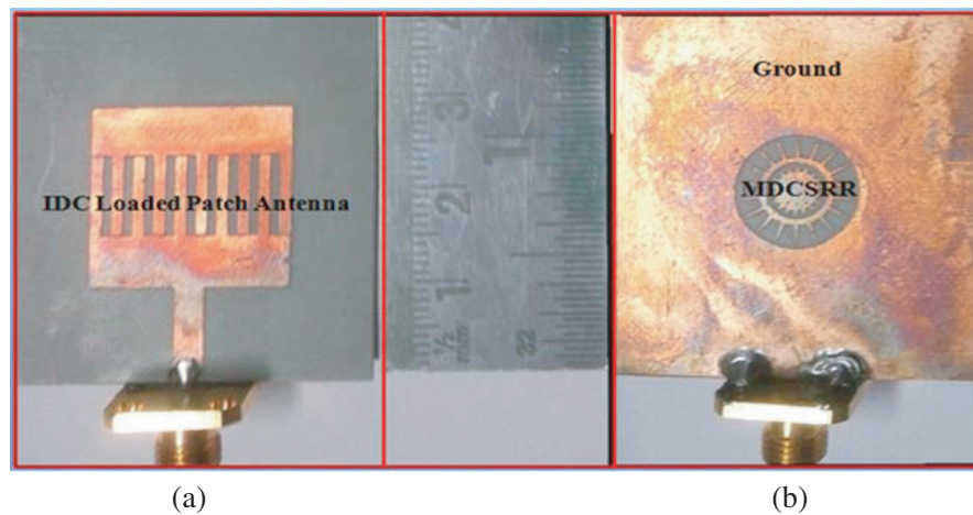
Figure 12. Fabricated MDCsRR metamaterial unit cell loaded microstrip patch antenna. (a) Top View and (b) back View.
