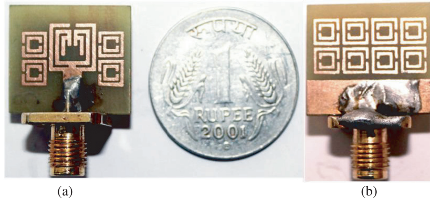
Figure 12. Fabricated prototypes (a) top (patch) and (b) bottom (ground) of Antenna 2 (considering stage 1).
