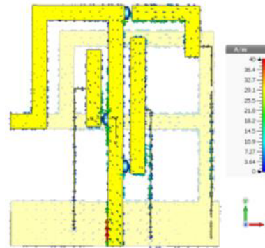
Figure 20. Surface current for case 7 (111) at 2.6 GHz.
