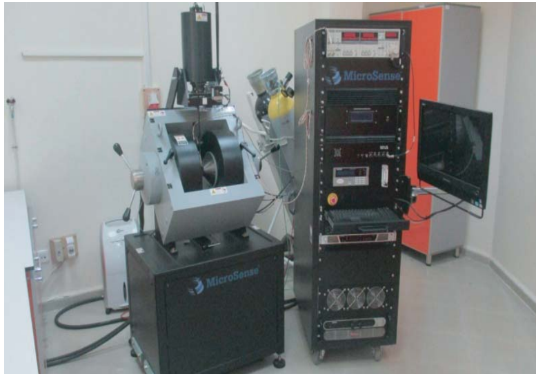
Figure 2. Vibrating sample magnetometer (VSM).
