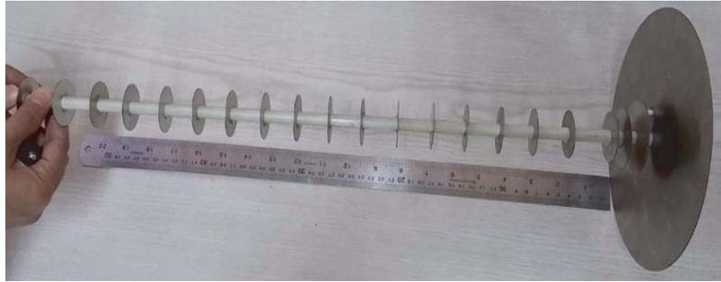
**Figure 7.** Manufactured prototype antenna with  $n = 17$  directors; Total length of the antenna is 510 mm.
