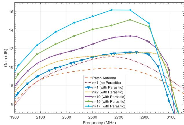
**Figure 5.** Simulated antenna gain versus frequency for *n* directors, the effect of the parasitic elements on the antenna gain is also illustrated.
