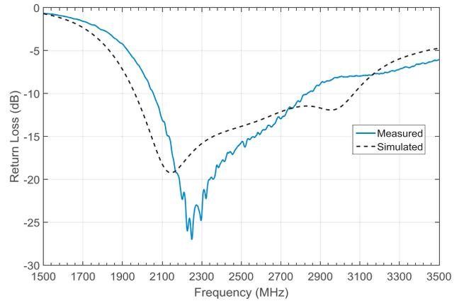
**Figure 2.** Measured and simulated *S*-parameter of the patch antenna.
