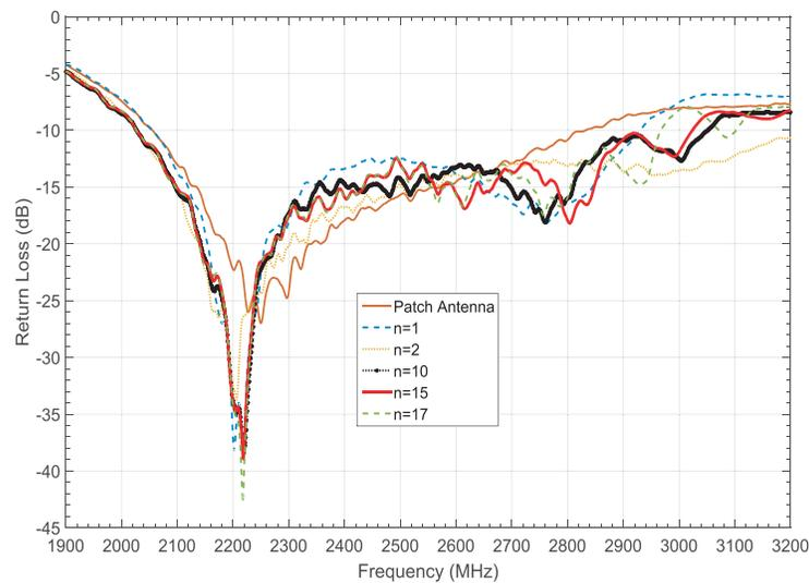
**Figure 8.** Measured return loss versus frequency for the patch antenna and the antenna with  $n$  directors including the parasitic elements.
