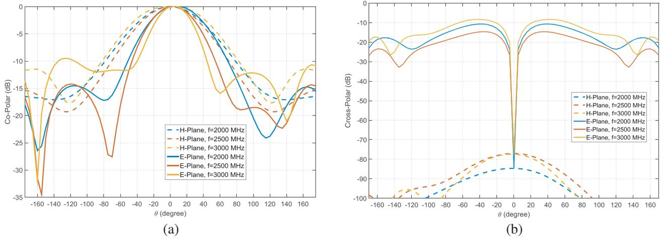
**Figure 3.** Simulated radiation pattern for *E*-plane and *H*-plane at 2000, 2500 and 3000 MHz. (a) Co-polar pattern, (b) cross-polar pattern.
