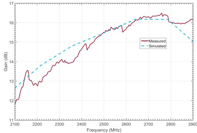
**Figure 10.** Measured and simulated antenna gain with  $n = 17$  directors.
