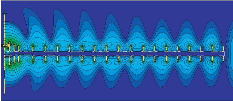
**Figure 6.** Contour plot of the electric field intensity at 2500 MHz. The high field intensity at the circular patch rims are visible and the field along the center of the circular patches is very small that is negligible which leads to an effective use of a dielectric rod as a mechanical holder.
