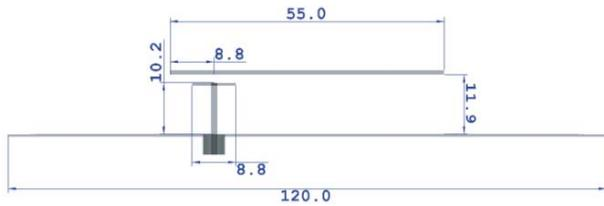
**Figure 1.** Side view of the circular patch antenna; The patch antenna is fed via a coupled feed disc on top of a circular ground plane.
