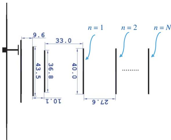
**Figure 4.** Patch antenna with *N* directors and two parasitic patches for impedance and gain adjustments. The distance among the directors are constant.
