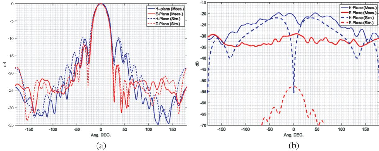
**Figure 9.** Measured and simulated co-polar and cross-polar radiation pattern of the antenna with  $n = 17$  directors at 2500 MHz.
