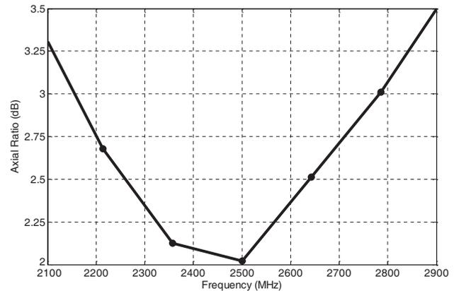
**Figure 12.** Simulated axial ratio (dB) versus frequency of the dual feed antenna geometry with 90 degree phase shifter.
