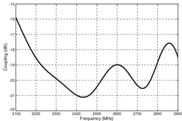
**Figure 11.** Simulated coupling (dB) between the two 90 degree physically rotated feeds versus frequency in the dual feed antenna geometry.
