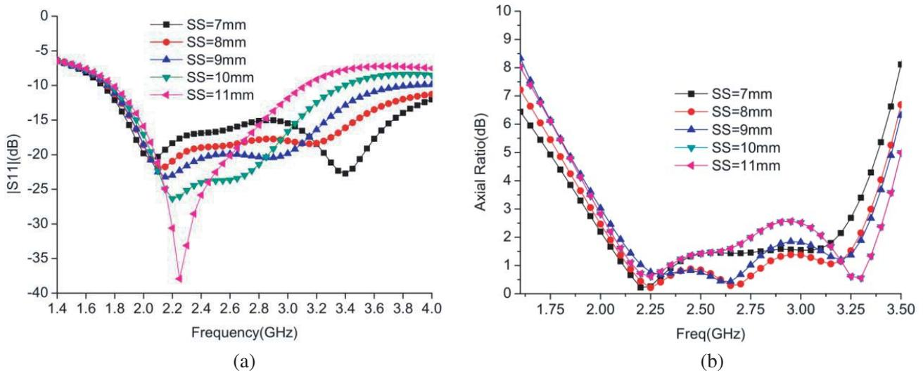
**Figure 7.** (a) Simulated  $|S_{11}|$  pattern for various  $SS$ . (b) Simulated AR pattern for various  $SS$ .
