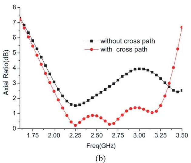
Figure 6. (a)  $|S_{11}|$  patterns for antennas with and without cross patch. (b) AR patterns for antennas with and without cross patch.
