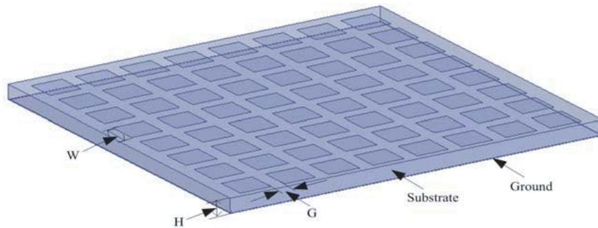
**Figure 1.** The AMC structure.
