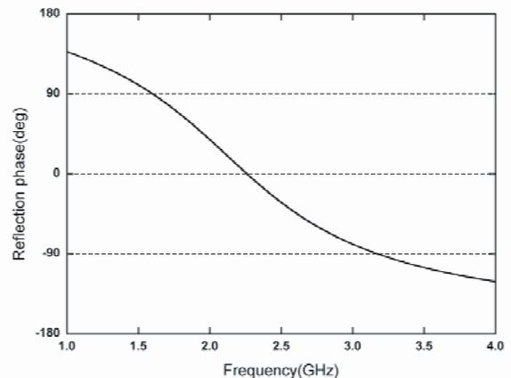
**Figure 3.** Reflection phase diagram of AMC structure.
