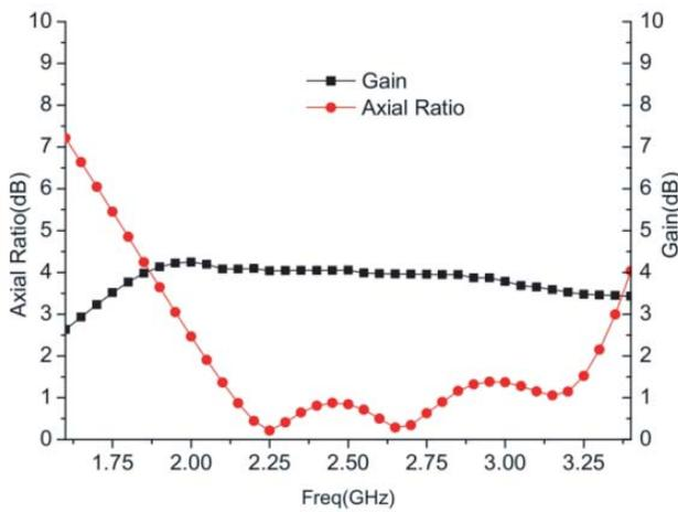
**Figure 9.** Gain and axial ratio of antenna.
