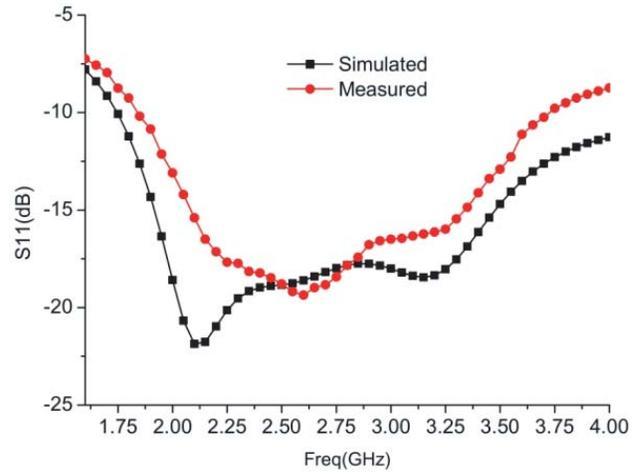
**Figure 10.** Measured and simulated  $|S_{11}|$  results.
