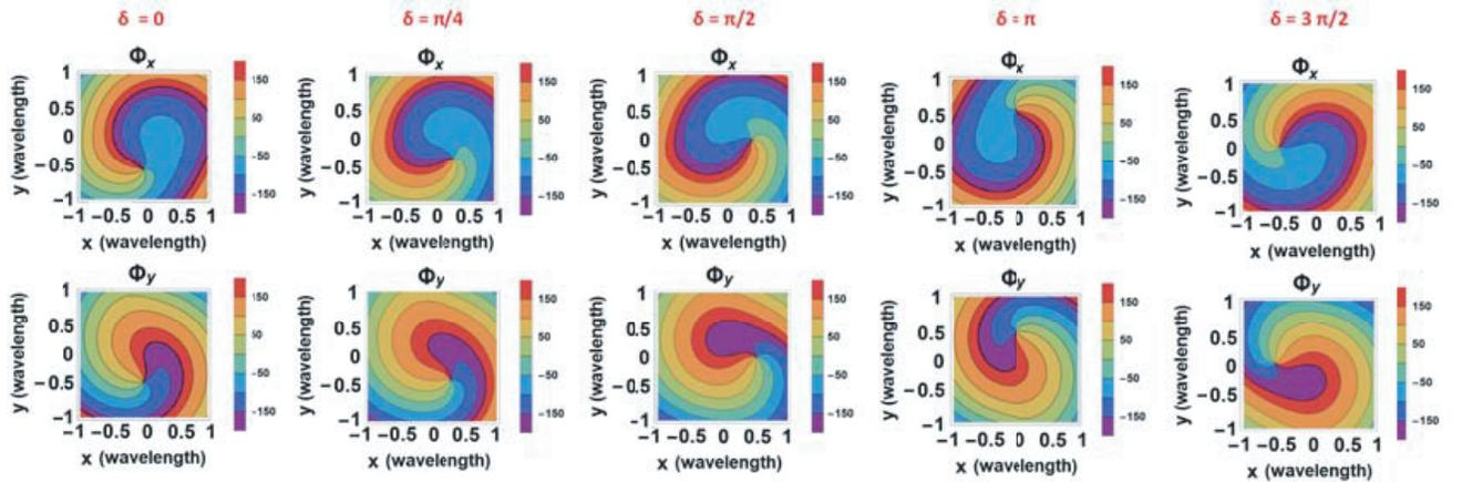
**Figure 3.** Analytically calculated phase ( $\Phi_x$  and  $\Phi_y$ ) distributions (in degree) of the electric field radiated by the superposition of RHCP  $\text{TM}_{11}$  and RHCP  $\text{TM}_{21}$  modes for different values of  $\delta$  (here  $\alpha = \frac{\pi}{4}$ ).
