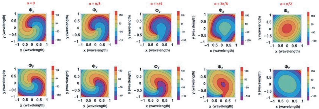
**Figure 1.** Analytically calculated phase ( $\Phi_x$  and  $\Phi_y$ ) distributions (in degree) at a distance  $\lambda_0$  from the patch of the electric field radiated by the superposition of RHCP  $TM_{11}$  and RHCP  $TM_{21}$  modes for different values of  $\alpha$  (here  $\delta = 0$ ).
