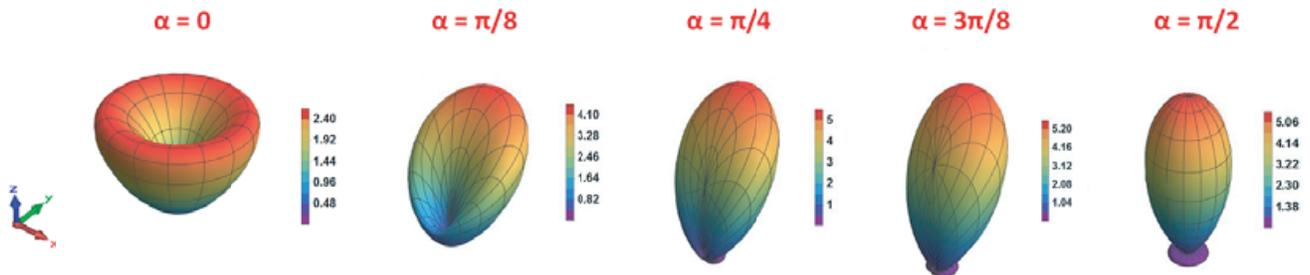
**Figure 5.** Analytically calculated directivity patterns (expressed in dB) of the patch antenna supporting the superposition of RHCP  $TM_{11}$  and RHCP  $TM_{21}$  modes for different values of  $\alpha$ .
