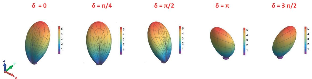
**Figure 6.** Analytically calculated directivity patterns (expressed in dB) of the patch antenna supporting the superposition of RHCP  $TM_{11}$  and RHCP  $TM_{21}$  modes for different values of  $\delta$ .
