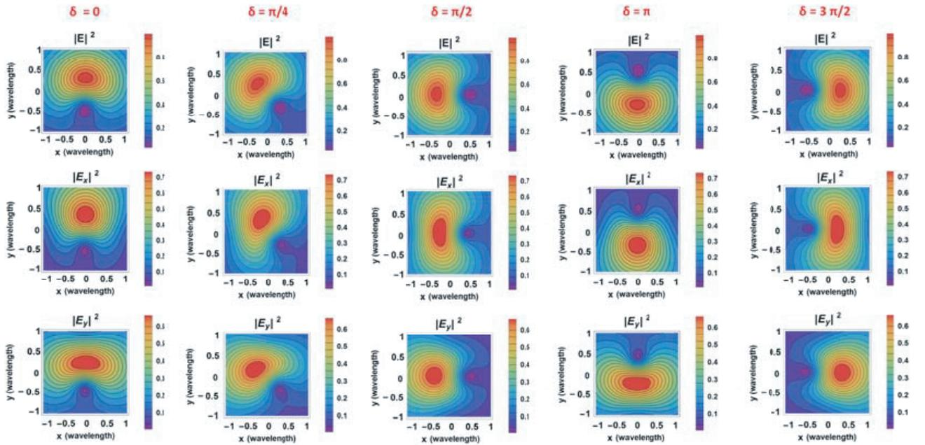
**Figure 4.** Analytically calculated total electric energy density ( $|E|^2$ ) and amplitude ( $|E_x|^2$  and  $|E_y|^2$ ) distributions of the electric field radiated by the superposition of RHCP  $\text{TM}_{11}$  and RHCP  $\text{TM}_{21}$  modes for different values of  $\delta$ .
