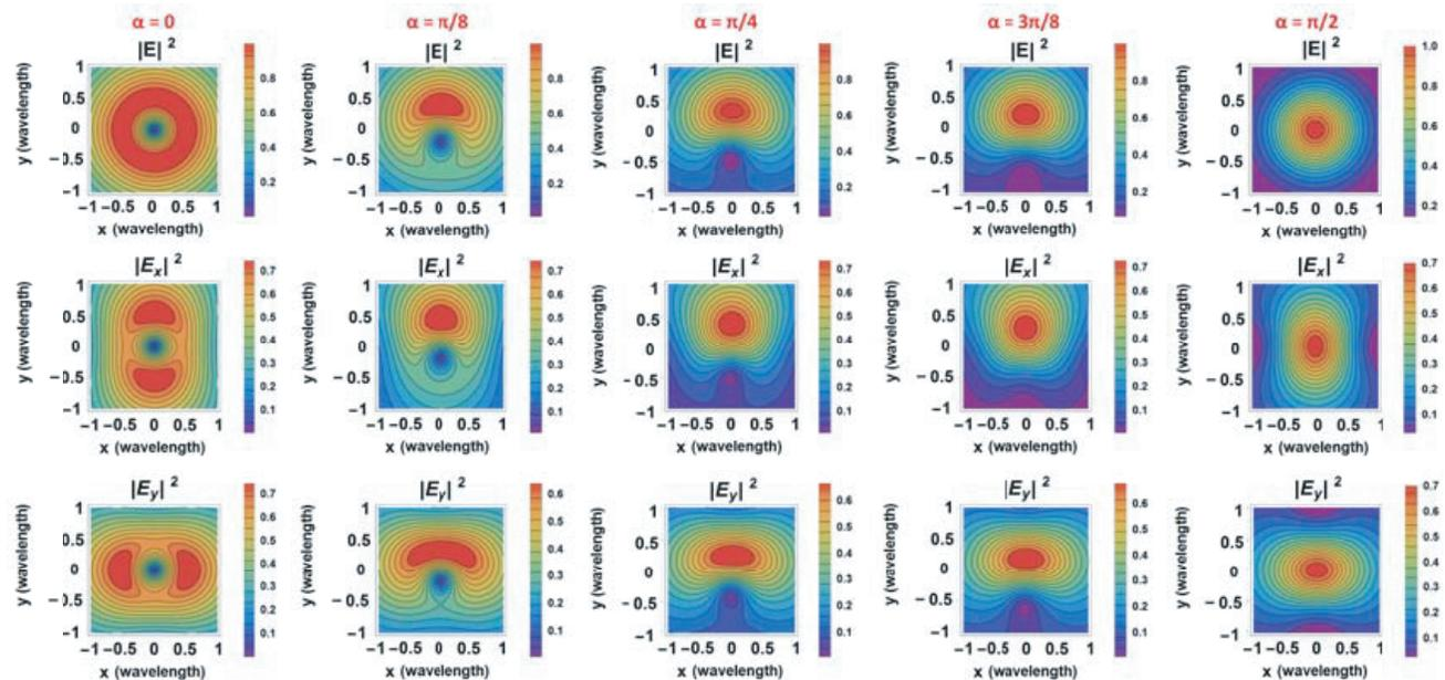
**Figure 2.** Analytically calculated total electric energy density ( $|E|^2$ ) and amplitude ( $|E_x|^2$  and  $|E_y|^2$ ) distributions of the electric field radiated by the superposition of RHCP  $TM_{11}$  and RHCP  $TM_{21}$  modes for different values of  $\alpha$ .
