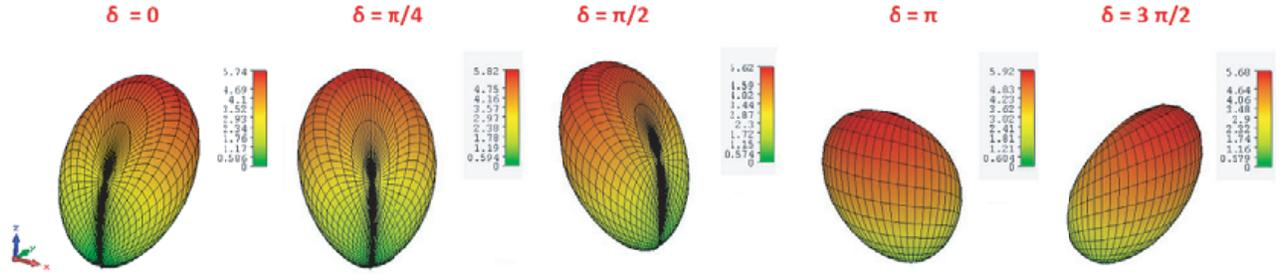
**Figure 12.** Numerically calculated gain patterns (expressed in dB) of the patch antenna supporting the superposition of a RHCP  $TM_{11}$  and a RHCP  $TM_{21}$  modes for different values of  $\delta$ .
