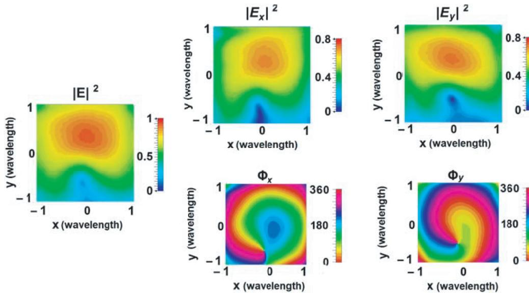
**Figure 10.** Numerically simulated total electric energy density ( $|E|^2$ ), amplitude ( $|E_x|^2$ ,  $|E_y|^2$ ) and phase ( $\Phi_x$ ,  $\Phi_y$ ) distributions of the electric field radiated by the proposed structure when excited with both a RHCP  $TM_{11}$  and a RHCP  $TM_{21}$  modes for  $\alpha = \pi/4$  and  $\delta = 0$ .
