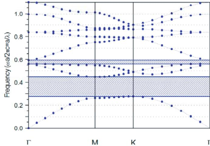
**Figure 1.** Band structure of triangular lattice photonic crystal of TM polarized light.
