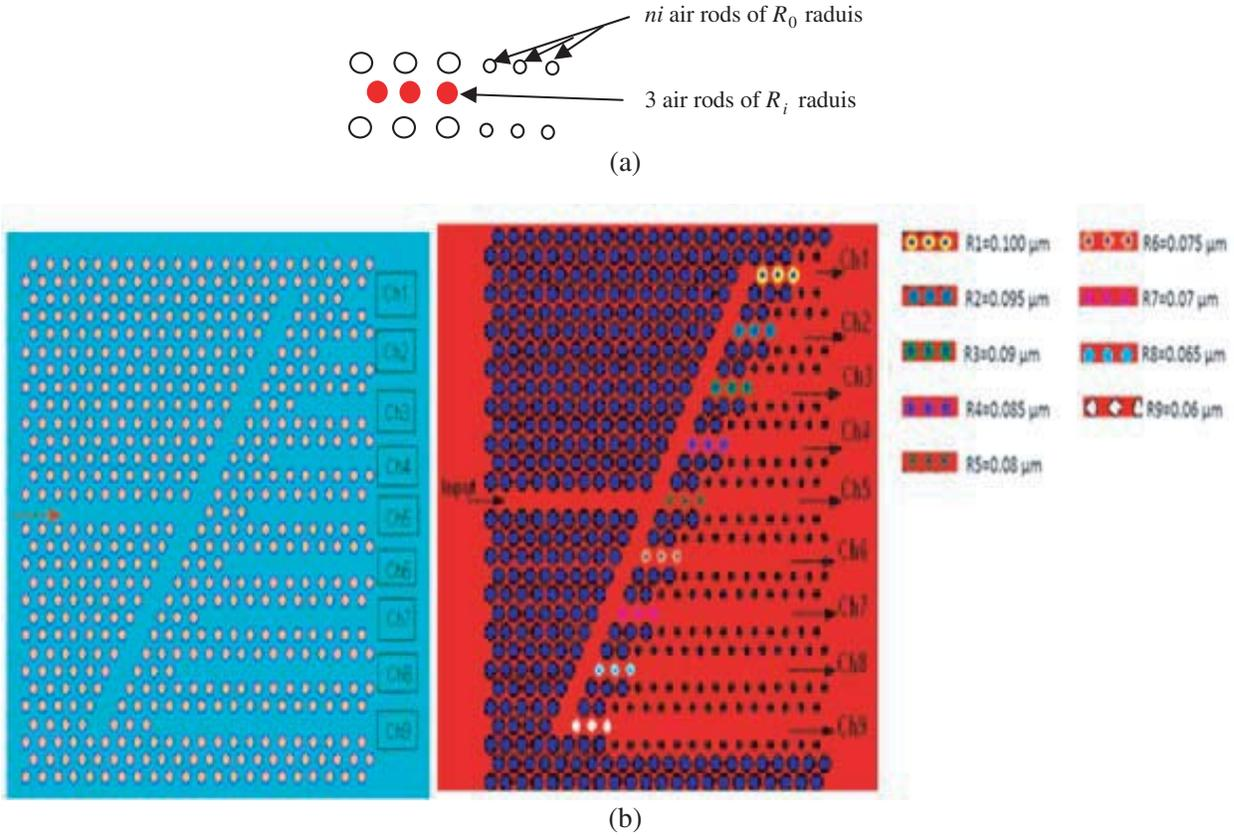
**Figure 2.** (a) Schematic diagram of the proposed defective resonant cavity. (b) Simulated structure.
