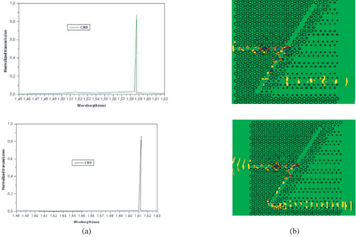
**Figure 3.** (a) Output spectral nine channel transmission separately. (b) Distribution of the magnetic field Hz separatel.
