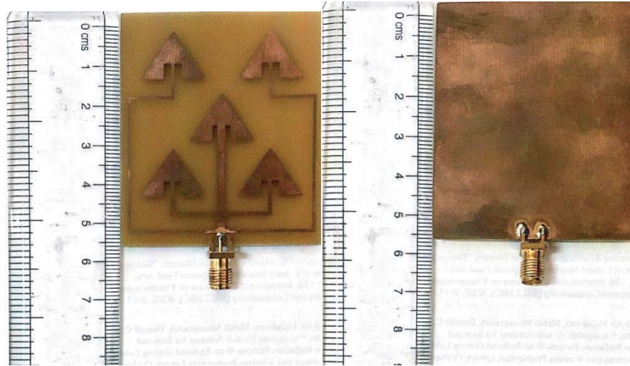
Figure 8. Prototype of realized antenna array.
