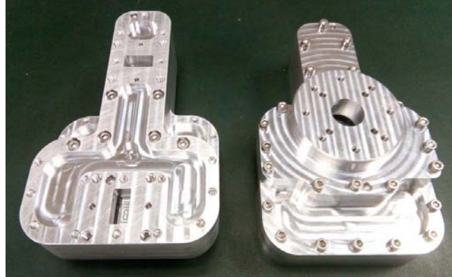
Figure 9. OMT platelet prototypes. skip0.1in
