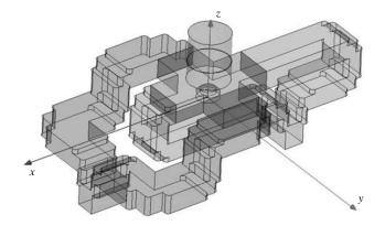
Figure 2. Hybrid OMT's design.
