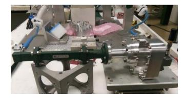
Figure 10. OMT measurement setup.
