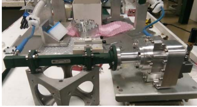
Figure 10. OMT measurement setup.
