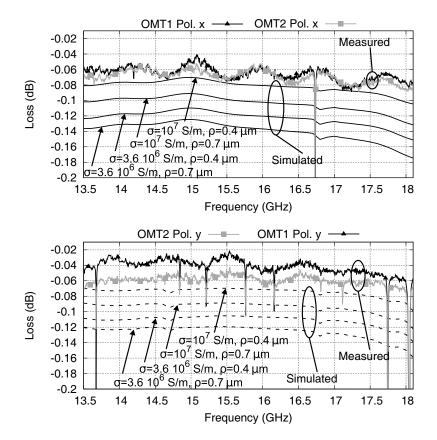
Figure 8. Hybrid model simulated and measured loss: top, x-polarization, bottom y-polarization.
