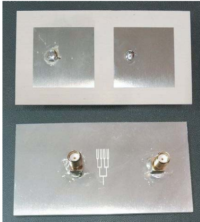
Figure 10. The fabricated antenna array with the Y shaped FDGS.
