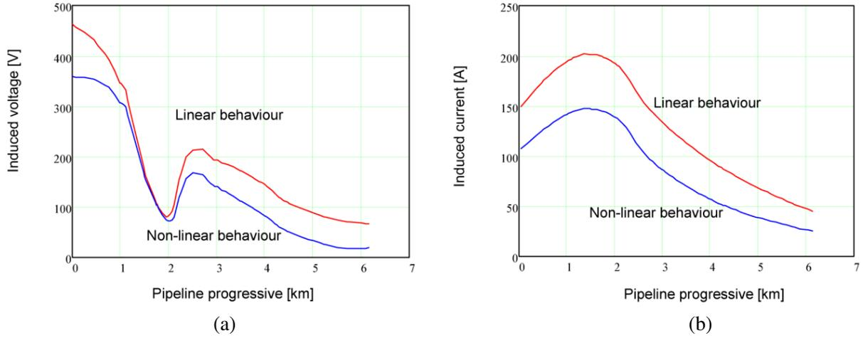
**Figure 4.** Comparison between the results of interference when taking into account or not the steel non-linearity effect.  $R_{ins} = 3 \cdot 10^6 \Omega\text{m}^2$ ,  $R_e = 5 \Omega$ . (a) Induced voltage. (b) Induced current.
