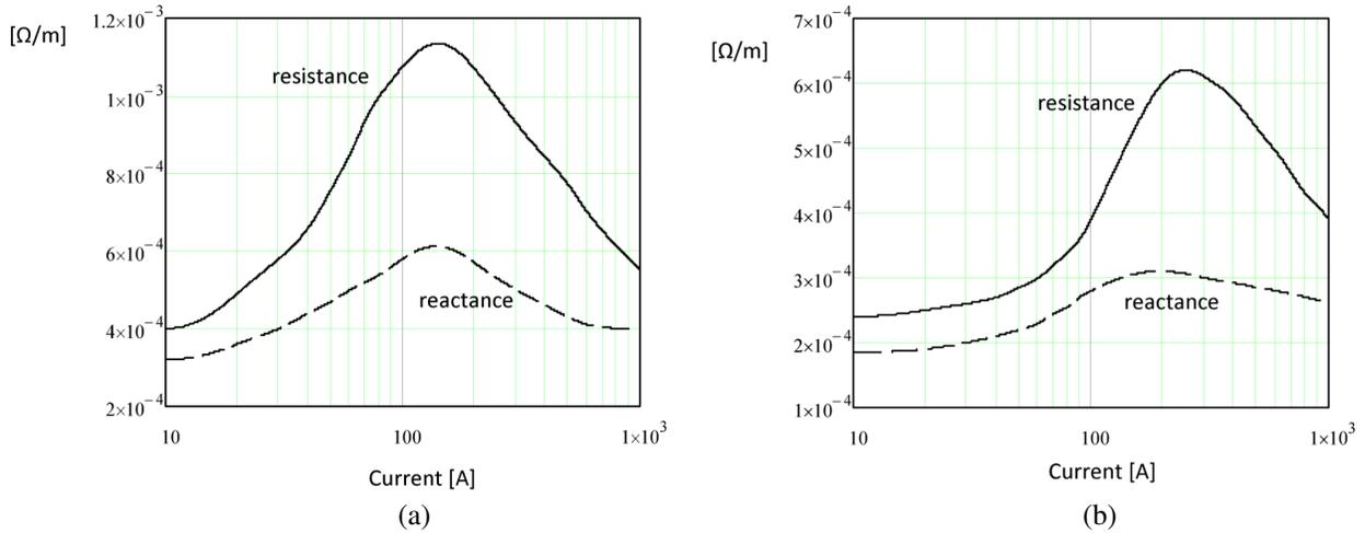
**Figure 1.** Measured p.u.l. internal impedance of a steel pipe versus the current;  $f = 50$  Hz. (a) 80 mm diameter, (b) 160 mm diameter.
