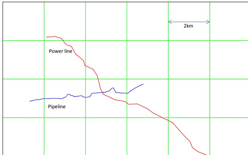
**Figure 3.** Lay-out of inducing power line and induced pipeline.
