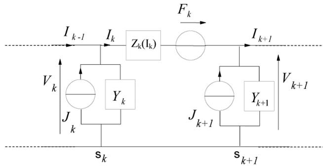
**Figure 2.**  $k$ -th  $\pi$  cell of the equivalent circuit modelling the pipeline with earth return.
