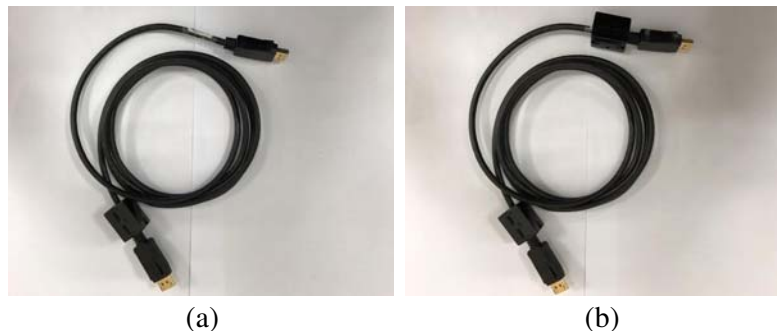
Figure 3. Signal line with added immunity magnetic ring. (a) 1 core. (b) 2 cores.
