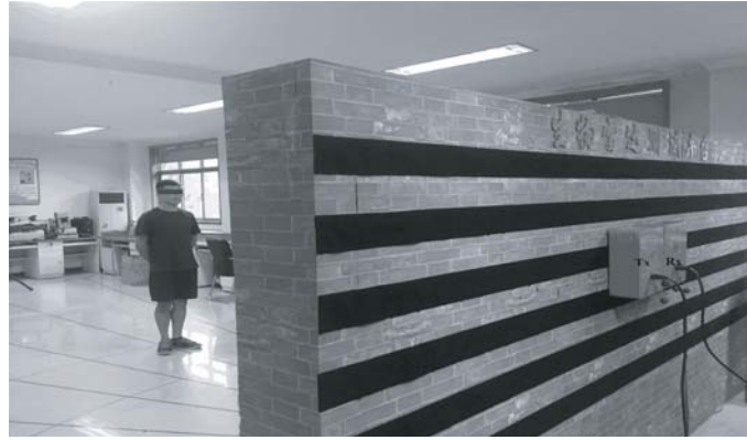
Figure 4. Experiment scenario of human respiratory signal detection based on IR-UWB radar, Tx is transmitting antenna, Rx is receiving antenna.
