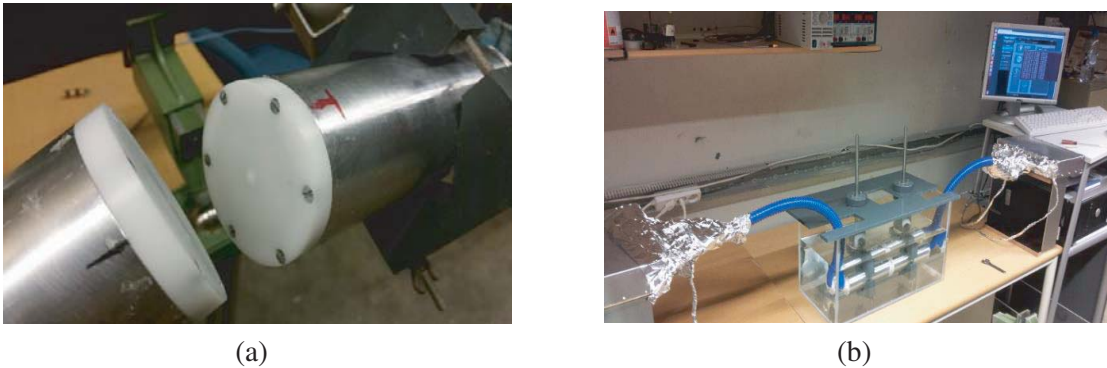
Figure 2. Lab setup: aluminum connectors where antennas were installed in (a), and overview of the measurement system (b).
