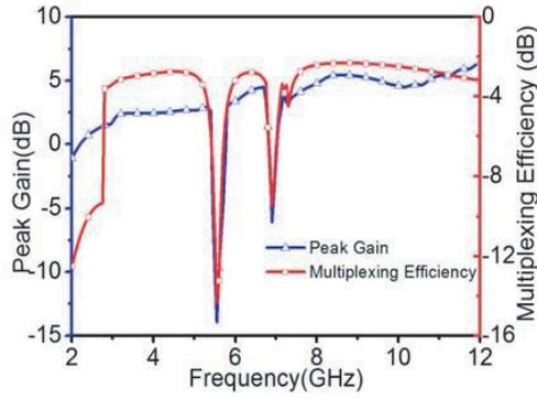
**Figure 11.** Multiplexing efficiency and Peak gain of the proposed antenna.
