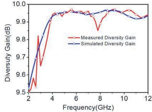
**Figure 10.** Simulated and measured DG values versus frequency of the proposed antenna.
