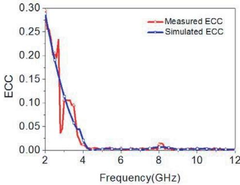
**Figure 9.** Simulated and measured ECC values versus frequency of the proposed antenna.
