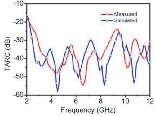
**Figure 12.** Simulated and measured TARC of the proposed antenna.
