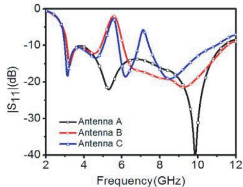
**Figure 3.** Simulated  $|S_{11}|$  of Antenna A, B and C.
