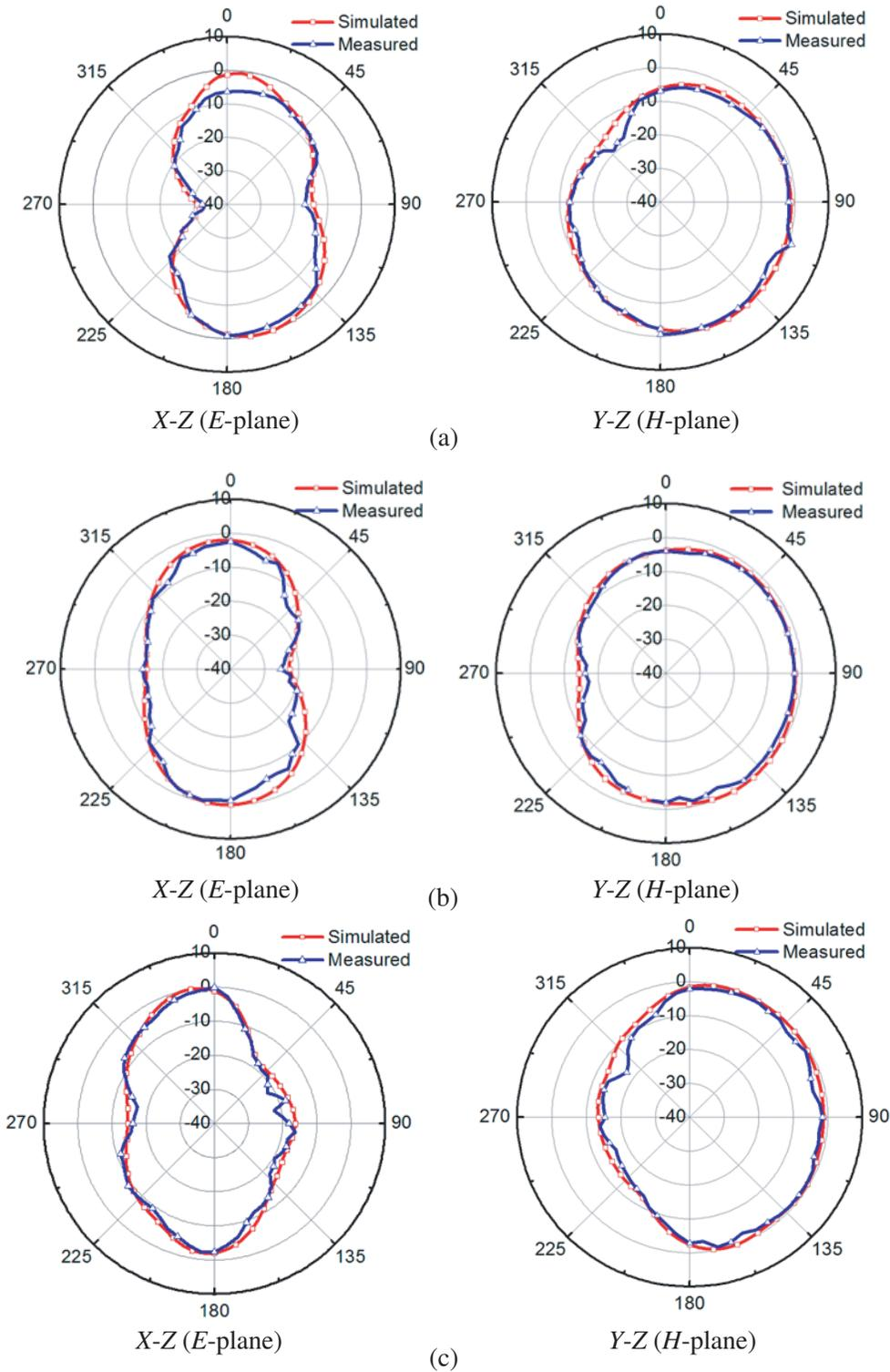
**Figure 8.** Simulated and measured radiation patterns of the proposed antenna. (a) 3 GHz. (b) 6.5 GHz. (c) 10 GHz.
