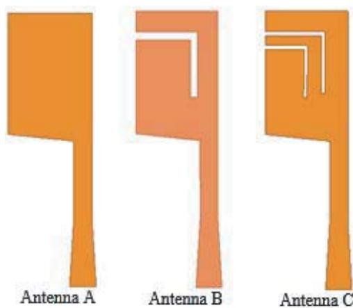
**Figure 2.** Configurations of the prototypes of Antenna A, B and C.
