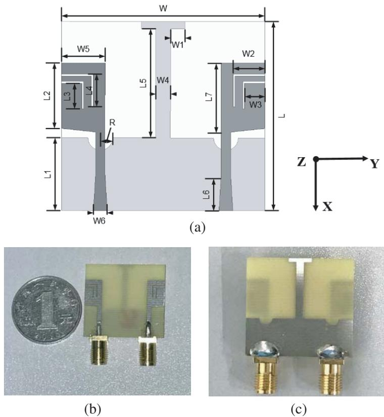
**Figure 1.** Proposed antenna geometry. (a) Structure of the proposed antenna. (b) Front view of the fabricated antenna. (c) Back view of the fabricated antenna.
