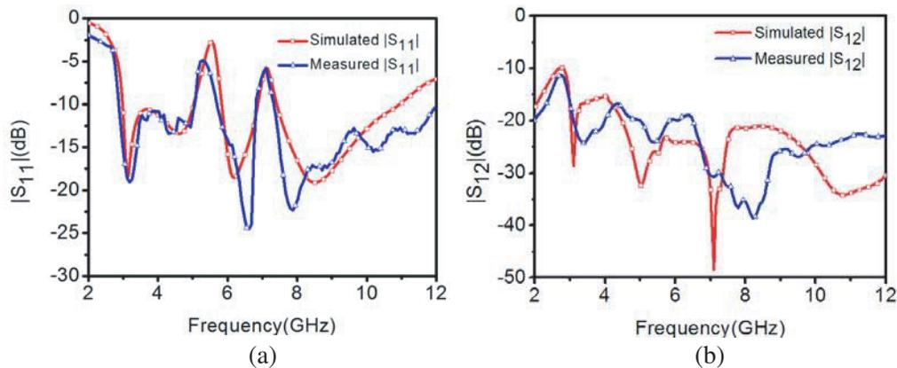
**Figure 7.** Simulated and measured  $S$ -parameters versus frequency of the proposed antenna. (a)  $|S_{11}|$ . (b)  $|S_{12}|$ .
