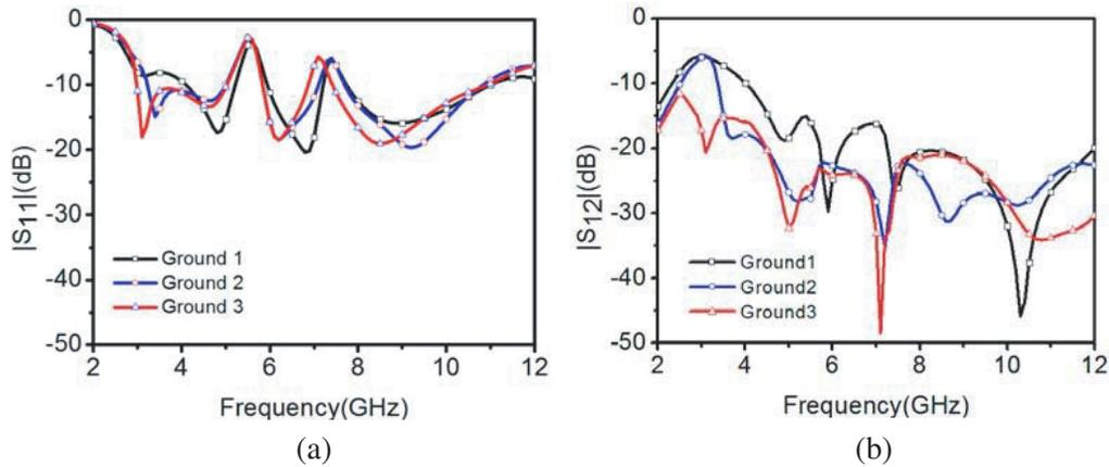
**Figure 6.** Simulated  $S$ -parameters of different ground planes. (a)  $|S_{11}|$ . (b)  $|S_{12}|$ .
