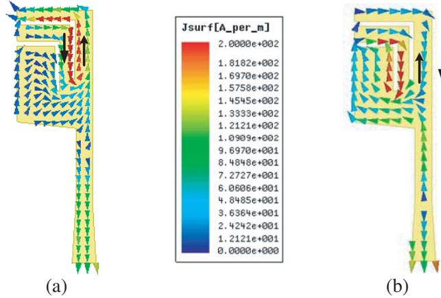
**Figure 4.** Simulated surface current distributions at different frequencies. (a) 5.5 GHz. (b) 6.9 GHz.
