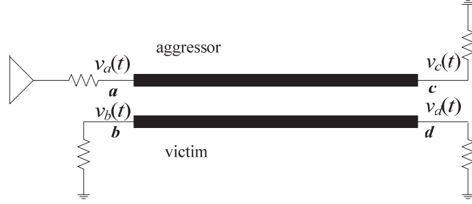
Figure 1. Crosstalk model between the microstrip transmission lines.
