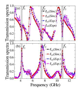
Figure 2. The simulated and measured (a) co-polarization  $(t_{xx} \text{ and } t_{yy})$  and (b) cross-polarization  $(t_{xy} \text{ and } t_{yx})$  transmission coefficients for the normal incident EM wave propagation along -z direction.
