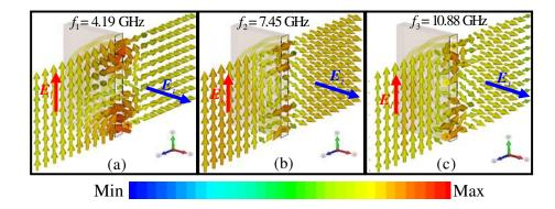
Figure 7. Simulated electric field distributions for the proposed PCMM in the case of the incident y-polarization wave along -z direction at different resonance frequencies: (a)  $f_1 = 4.19$  GHz, (b)  $f_2 = 7.45$  GHz, (c)  $f_3 = 10.88$  GHz. Bold arrows qualitatively indicate the direction strength of electric field.
