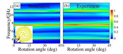
Figure 5. The (a) simulated and (b) measured cross-polarization transmission coefficient  $(t_{xy})$  of the proposed PCMM with different polarization angle  $(\varphi)$  of the incident electric field respect to the y-axis.
