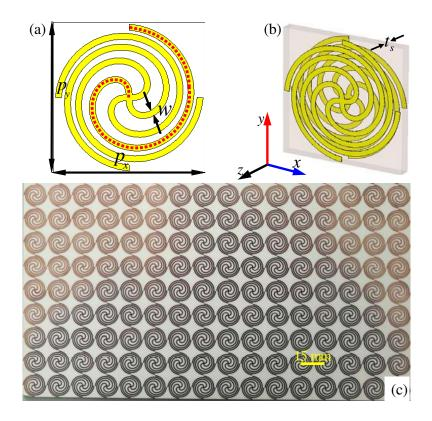
**Figure 1.** (a), (b) The front view and perspective view of the unit-cell structure of the designed PCMM, (c) a portion of photograph of the fabricated sample.
