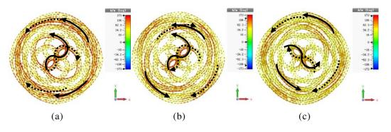
Figure 6. The simulated surface currents distributions of the unit-cell structure for the proposed PCMM in the case of incident y-polarized wave propagating along -z direction at (a)  $f_1 = 4.19$  GHz, (b)  $f_2 = 7.45$  GHz, (c)  $f_3 = 10.88$  GHz. The sold and dash line arrow indicate the surface current flow direction of the front and back layer structure.
