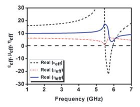
Figure 3. Effective permittivity ( $\varepsilon_{\text{eff}}$ ), permeability ( $\mu_{\text{eff}}$ ) and refractive index ( $\varepsilon_{\text{eff}}$ ) of proposed unit cell.
