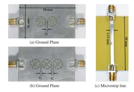
**Figure 8.** Fabricated prototype for (a) N = 2, (b) N = 3, (c) microstrip line.
