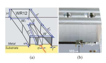
Figure 3. The geometrical parameters of the designed waveguide (WR12) to microstrip transition in (a), and the photograph of the fabricated prototype in (b).
