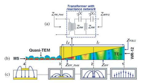
**Figure 5.** The metal ridge/substrate junction equivalent circuit in (a), simulated electrical field inside transition in (b), and the electric field intensity distributions at the main cross-sections (1–4) in (c).
