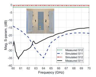
**Figure 4.** Simulated and measured *S*-parameters results of the fabricated back-to-back transition prototype over the frequency range of 60 GHz to 70 GHz.
