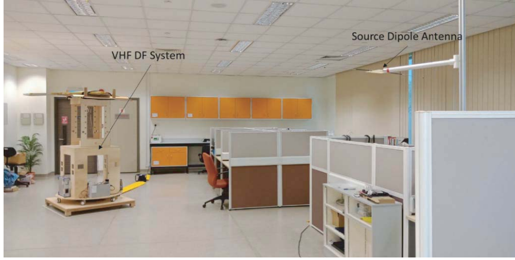
Figure 8. The Direction Finding test setup.
