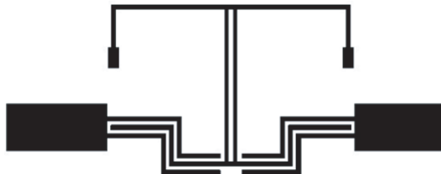
Figure 5. The proposed filter with meandering and stepped impedance open stub.
