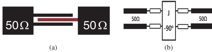
Figure 16. (a) Schematic and (b) equivalent transmission line network of the inter-digital coupled lines [13].
