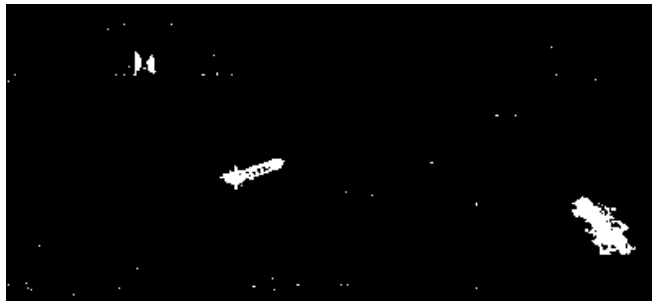
Figure 7. Detection result obtained with the Gamma-based CFAR detector.
