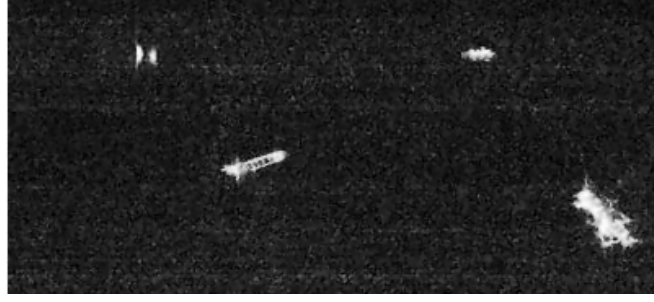
Figure 3. SAR image generated by using the GAN. One generated virtual target is at the top right corner.
