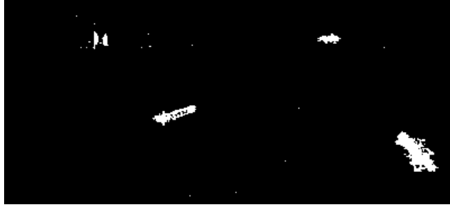
Figure 4. Initial result obtained with the Weibull-based CFAR detector.
